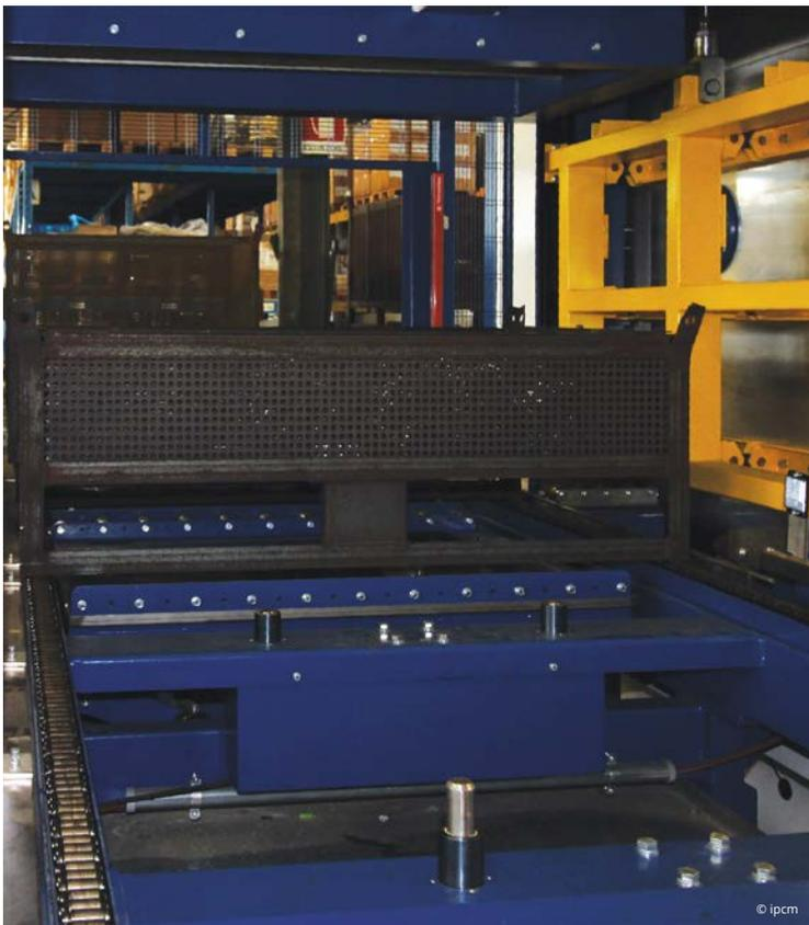
A basket being taken into the cleaning chamber by the automatic arm.
